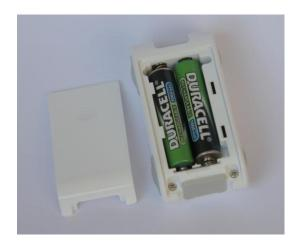
Rechargeable batteries are recommended, and you should make sure to recharge the batteries before each flight day. Tests have shown that the Flight Recorder will run for over 8 hours on standard 1000 mAh NiMH rechargeable batteries. After some time, the rechargeable batteries will lose capacity and it is recommended that you check the battery status during long flights.
