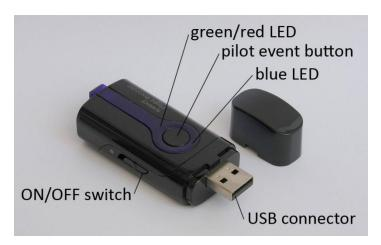
On the top of the device there is pilot event button. By pressing this button Flight Recorder will record an event which will be also saved in IGC file and will be displayed in IGC viewer. When pressing the button the blue LED will flash quickly.
